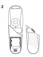
Match the + and – marks on the batteries to the + and – marks in the battery case, then insert the batteries.
